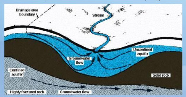
Confined: Upper boundary relatively impervious – groundwater under pressure. Level constant (but pressure varies)
